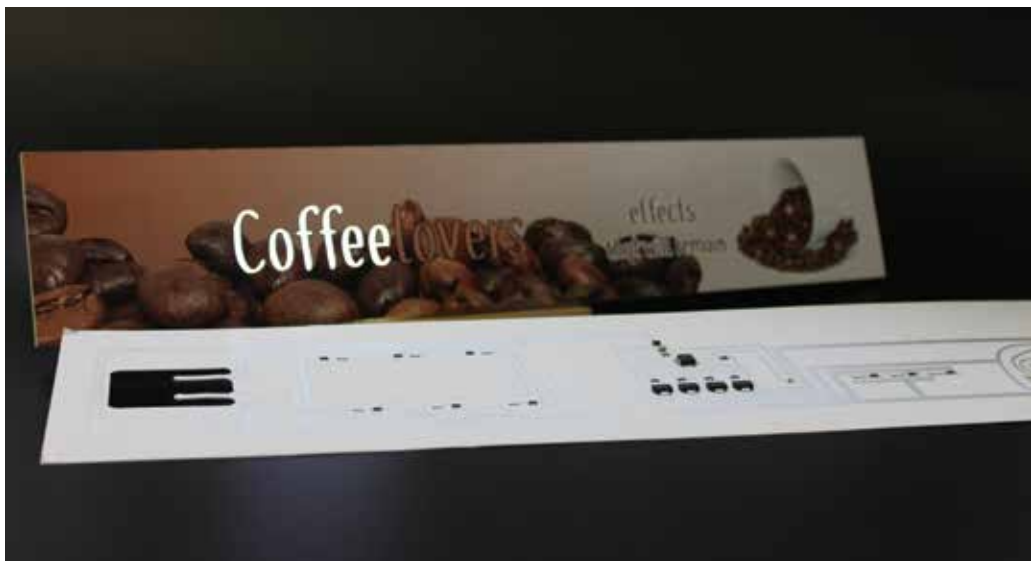
Figure 4: Hybrid printed electronics on paper with SMD components for illuminated PoS applications
