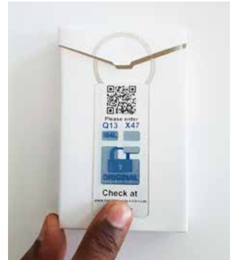
Figure 2: Integrated printing of batteries, electrochromic displays, a push button and graphic colour as a security sticker
